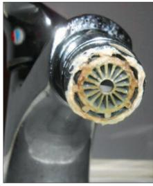
A heavily scaled plastic tap insert in an augmented care ward, which is also showing some evidence of biofilm.
