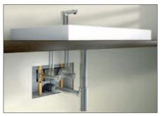
The Kemper HyTwin system allows water to recirculate up to and through the tap outlet, with the aim of further reducing environments for biofilm to develop.
