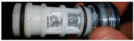
A TMV strainer with pipe joining compound, Boss White, accumulated on strainer mesh. Pseudomonas aeruginosa was recovered from this TMV strainer and many others within this particular system.
